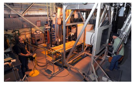
FCF includes a mock-up shop where technicians can build and test new hot cell equipment before installing it into the hot cell.
