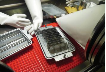
ZPPR operators performing material inspections in the transuranic surveillance glovebox.
