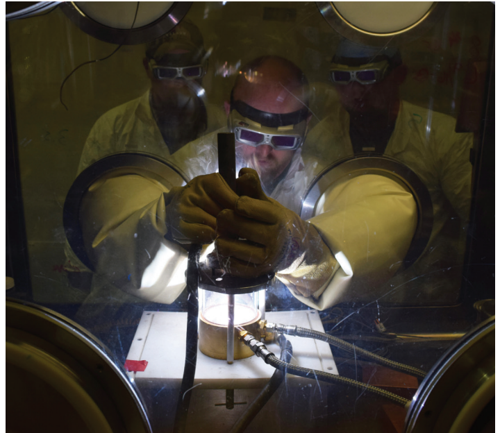
Arc melting in the Advanced Fuel Cycle Initiative (AFCI) glovebox supports fabrication of experiments for irradiation at reactors such as the Advanced Test Reactor.
