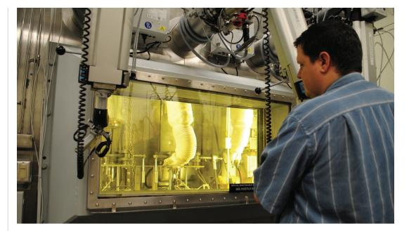
The Irradiation-Assisted Stress Corrosion Cracking hot cells are located in FASB's west room.
